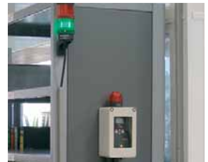
RadEye Area Monitor for neutron radiation
