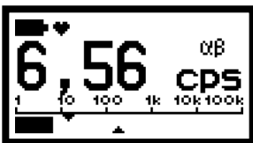
Simultaneous measurement of alpha, beta and gamma radiation
