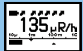
Approaching a source Alarm thresholds - not yet exceeded. Trend arrow indicates increasing radiation level
